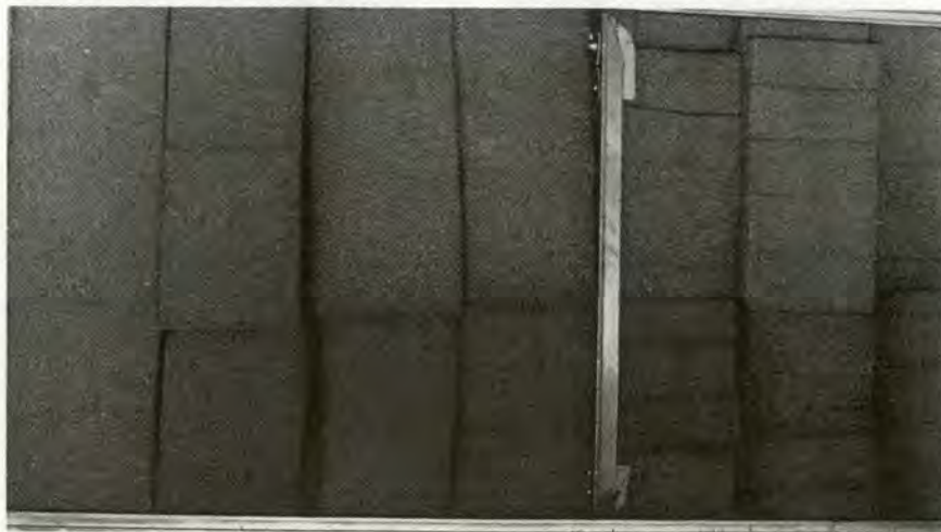
C-130 fuel tank with foam. All the foam must be installed. Removing part of the foam has led to fuel sloshing, static buildup, discharge and explosion.
