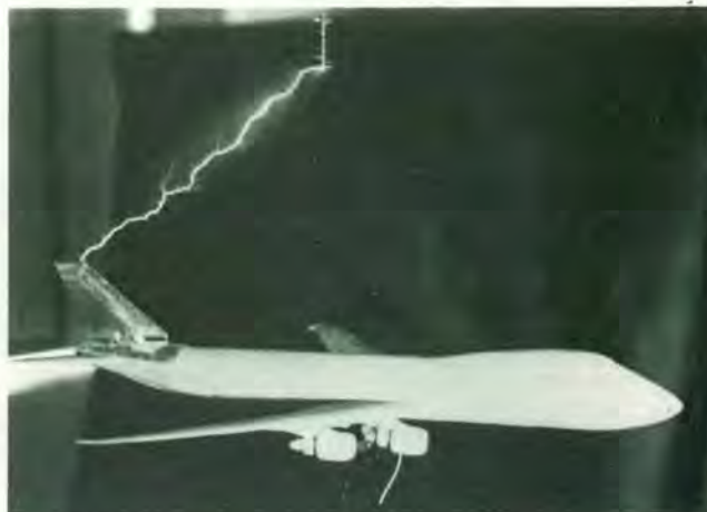
Figure 8B Long arc test on 747 model shows attachment to the vertical stabilizer.
