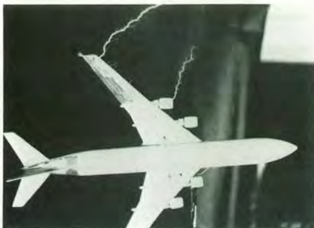
Figure 8A Long arc tests on 747 model show attachment on left wing and streamering from No. 1 nacelle.
