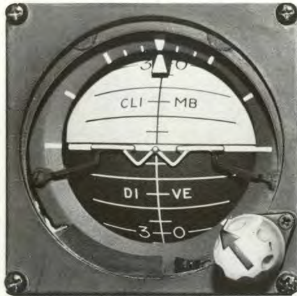
The F-16 SADI is a simple DC powered two axis mil standard gyro that might just save your life.
